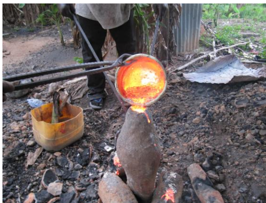
PLATE 3.63: Pouring molten metal into mould
