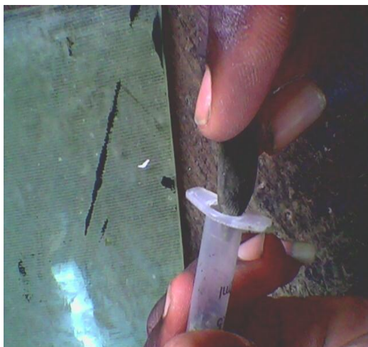
PLATE 3.30: Inserting wax into syringe
