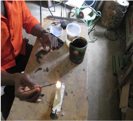
PLATE 3.22: Heating tool for wax build-up PLATE 3.23: Built-up pattern
