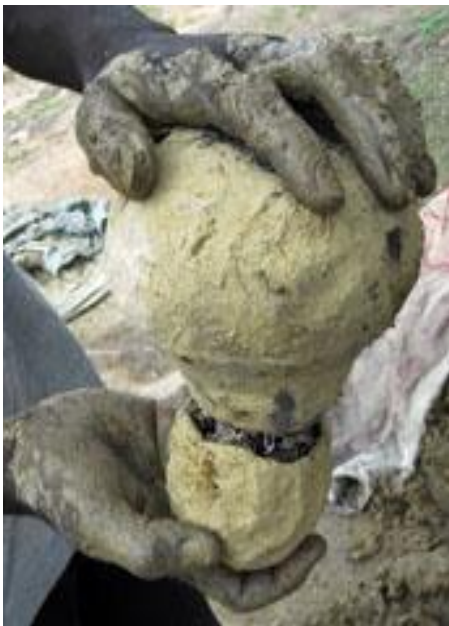
PLATE 3.58: Attaching crucible to mould
