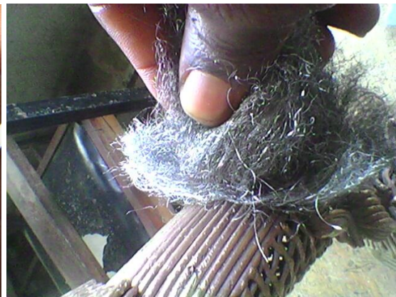
PLATE 3.68: Polishing with steel wool
