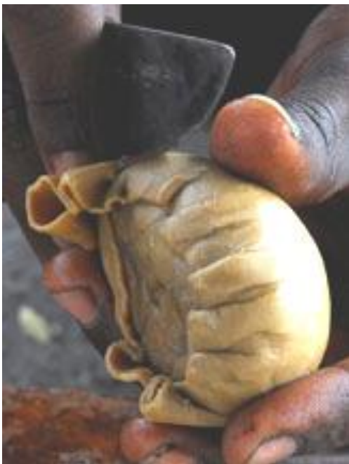
PLATE 3.27: Cutting wax from core
