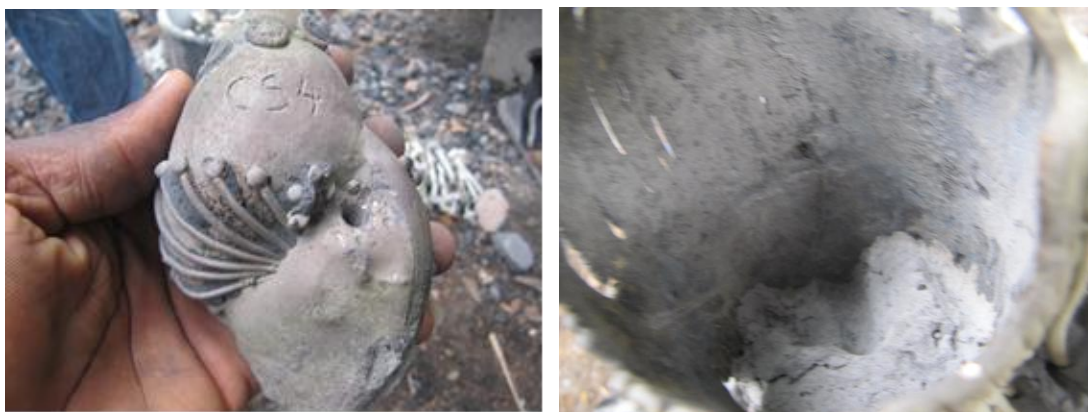
PLATE 3.47: Sample KCS4 after casting PLATE 3.48: Inner wall of sample cast item
