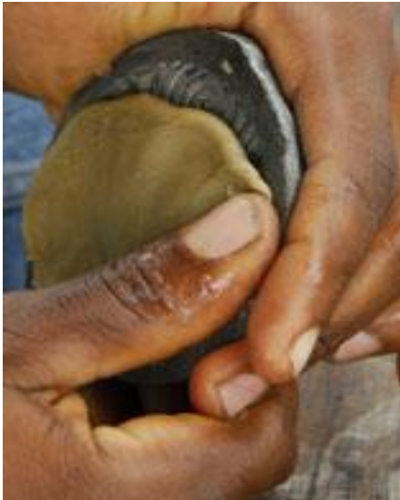
PLATE 3.8: Wax pressed into mould
