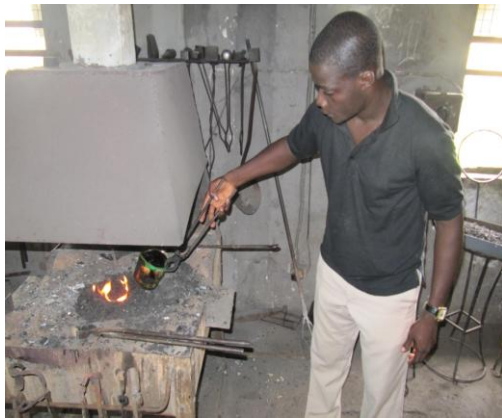
PLATE 3.12: Melting of wax
