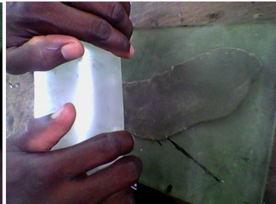
PLATE 3.38: Pressing to form sheet wax
