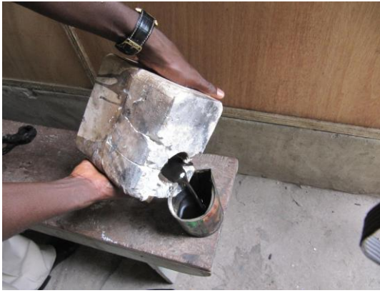
PLATE 3.16: Pouring wax from mould
