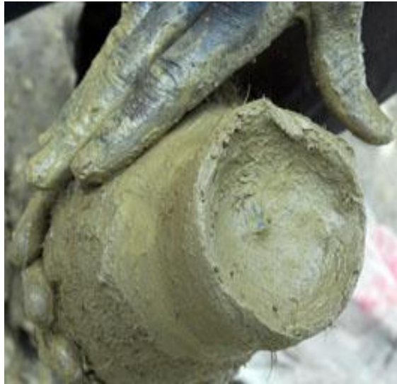
PLATE 3.57: Mould with palm fibre coating
