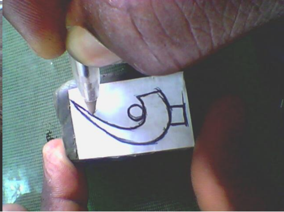
PLATE 3.19: Transferring design unto wax
