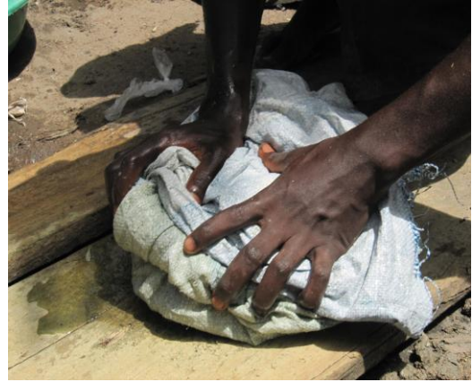
PLATE 3.66: Polishing in a sack
